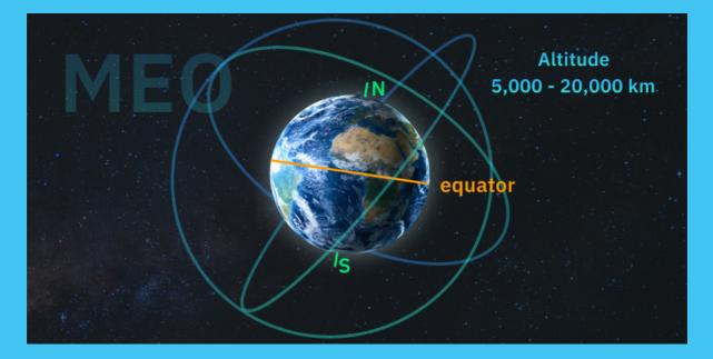
Medium Earth orbit comprises a wide range of orbits anywhere between LEO and GEO. It is similar to LEO in that it also does not need to take specific paths around Earth, and it is used by a variety of satellites with many different applications.
